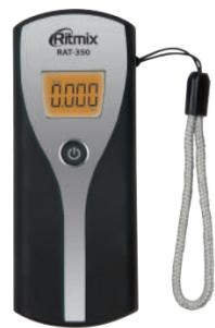
Thanks for purchasing Ritmix RAT-350 hand held Digital Alcohol Analyzer. Ritmix RAT-350 Alcohol tester is for making the personal test of measuring the alcohol in the exhaled vapor. Tester recalculates the data and provides the results as concentration of alcohol in blood.
